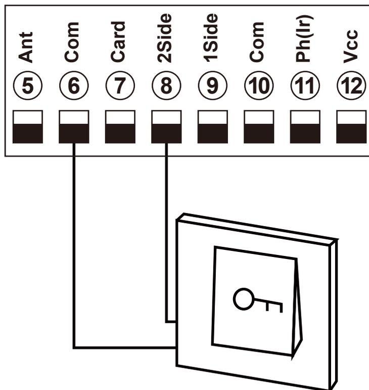
Terminal ⑧2SIDE and ⑥COM are use to connect with push button for controlling dual gates.
