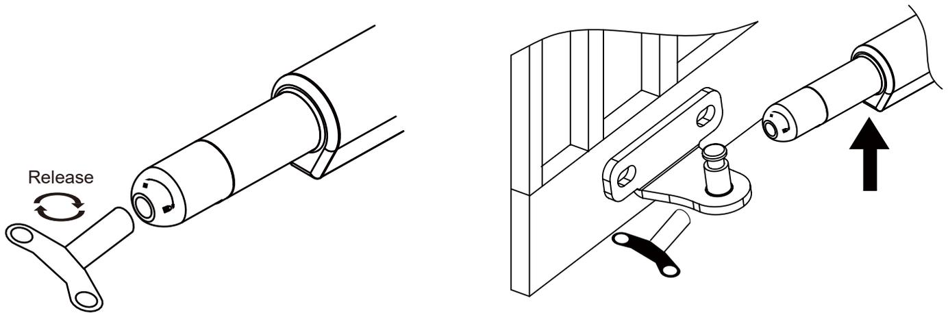
The schematic diagram of opening the gate body when there is no power is shown above. Please use the emergency release key to loosen the gate bracket and the arm of the gate opener. Then lift it up.
