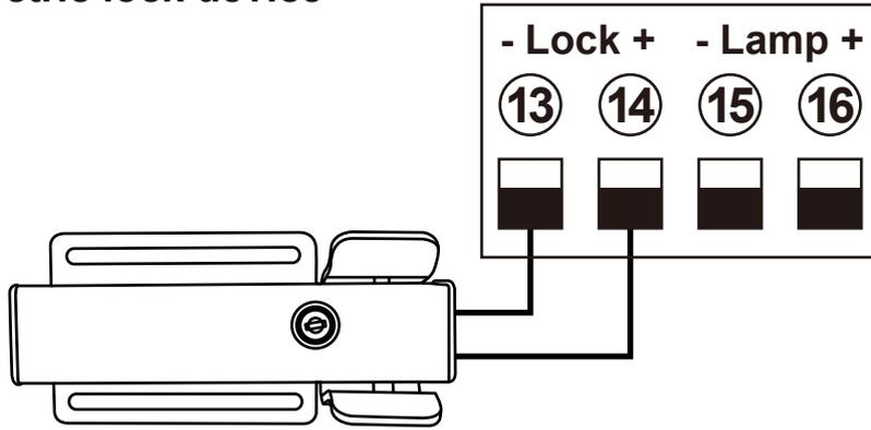
Terminal ⑬ LOCK- is used to connect with electric lock blue wire.
