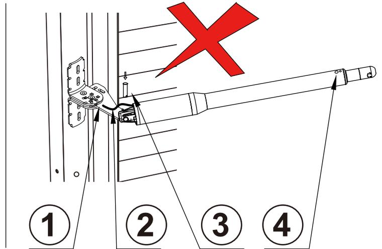
**Figure right, Power Cable And Rain Drainage Aperture Placed Incorrectly**
