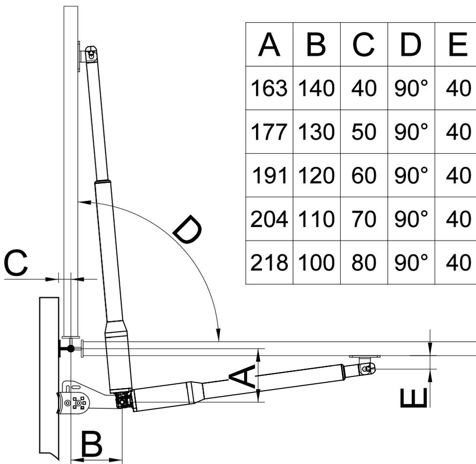
(1). According to the diagram, the post bracket plate is attached the fixed bracket with an appropriate angle. Take out the gate opener arm to install 2pcs Pivot Arc Bracket (H) and Post Pivot Bracket (J) on the gate post. Fig ① and ② are left bracket install instruction, ③ and ④ are right bracket install instruction.
