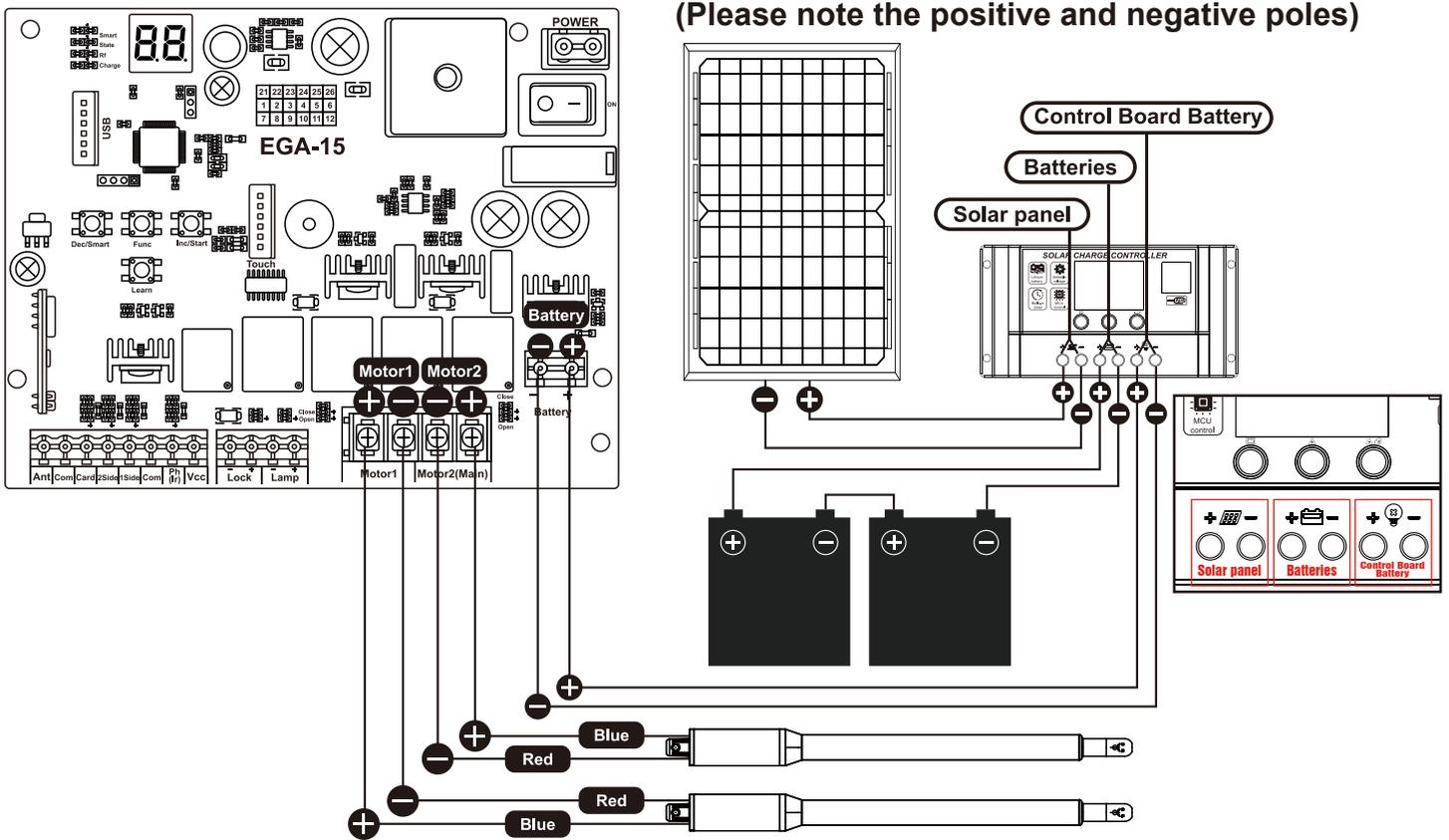
• Type 3: By AC Electricity, Solar Panels and Back-up Batteries (Solar panel, charger and batteries are not included)
