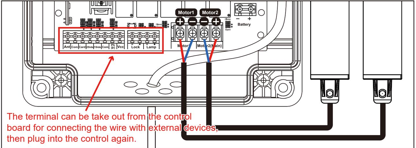
**Motor 1** Insert the stripped cable wires into the appropriate terminals on the opener terminal block. The red wire should be inserted into the “ **MOTOR 1 +** ” terminal, the blue wire into “ **MOTOR 1 -** ” terminal.
