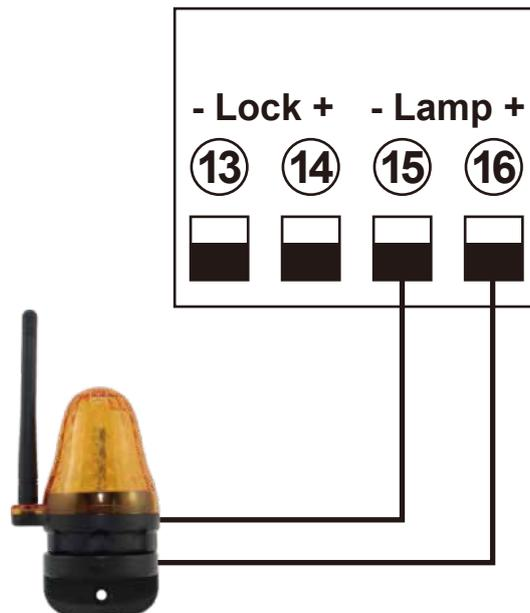
Terminal ⑮⑯Lamp + / - are used to connect with flash lamp.
