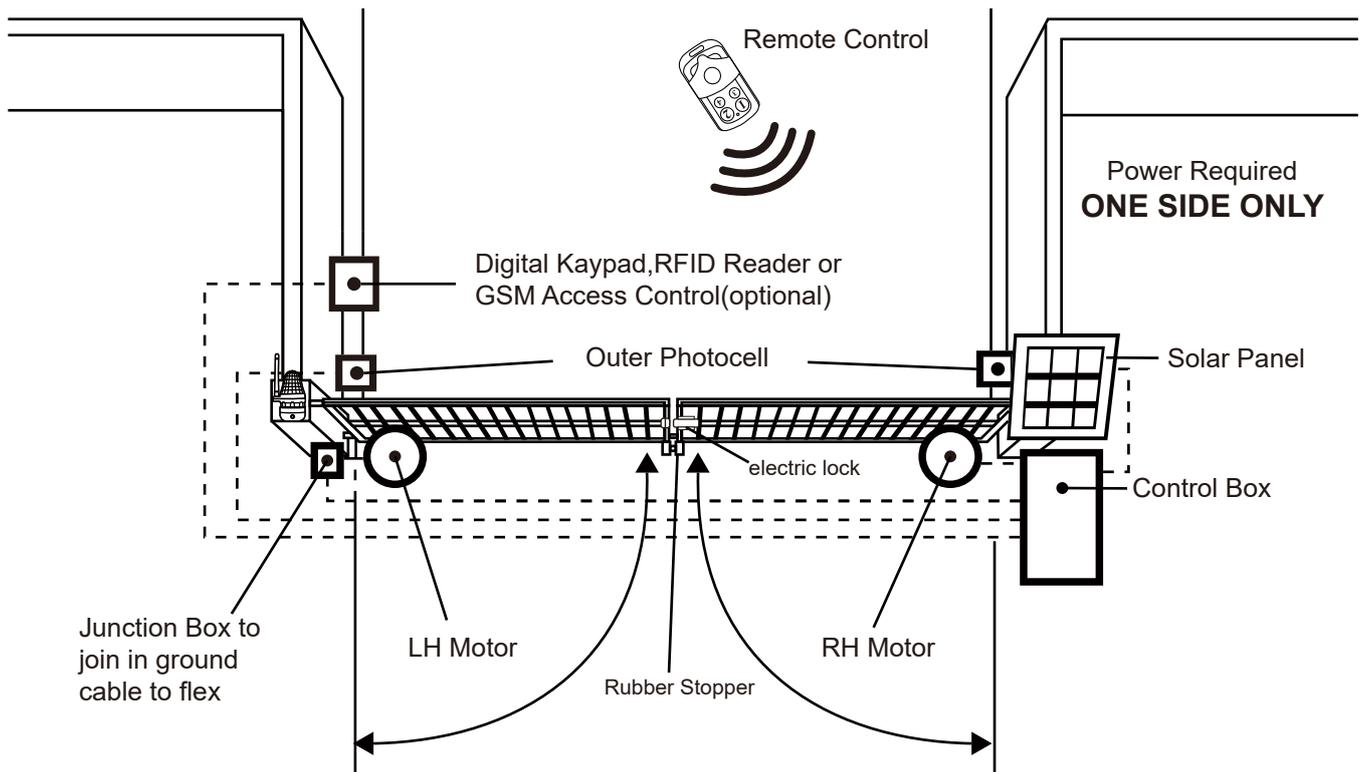
Photocell Beam System, Warning Sign, Flash Lamp, Solar Panel, Gate Opener (Gate 2) (Left), Electric Lock, Gate Opener (Gate 1) (Right), Rubber Stopper
