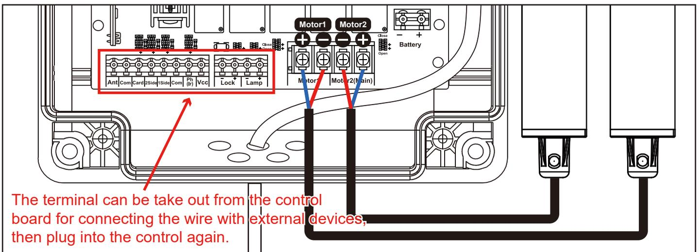
The terminal can be take out from the control board for connecting the wire with external devices, then plug into the control again.
