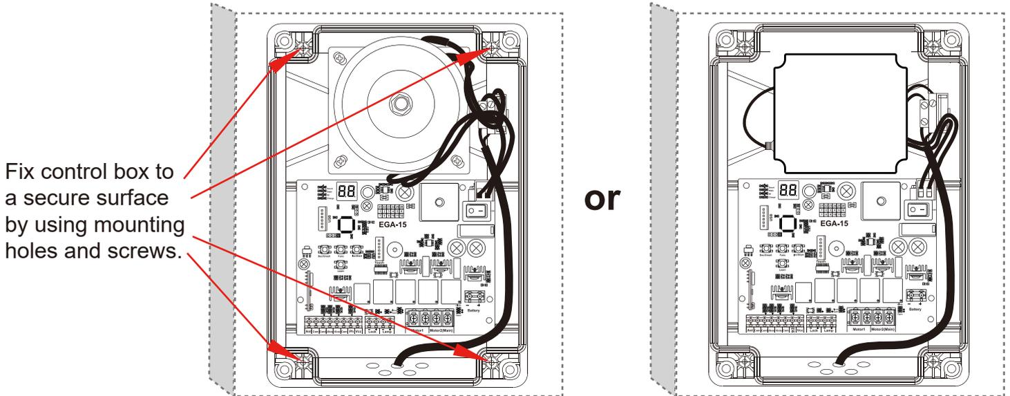
Fix control box to a secure surface by using mounting holes and screws.
