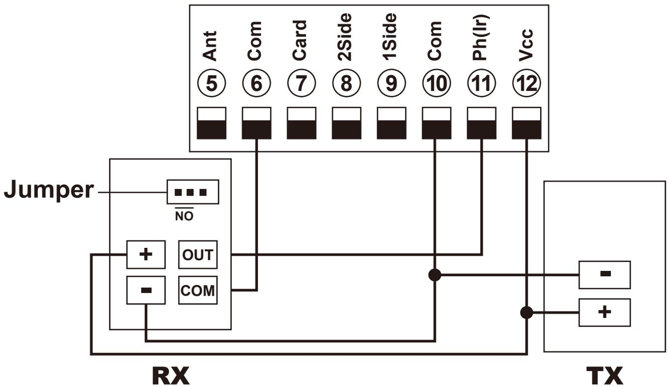
Terminal ⑫VCC and ⑩COM are used to supply power to safety beam sensor device. So, connect terminal ⑫VCC with the “+” of the safety beam sensor RX and TX device. Connect terminal ⑩ COM with the “-” of the safety beam sensor RX and TX device. Connect terminal ⑪PH(Ir) with safety beam sensor “OUT”
