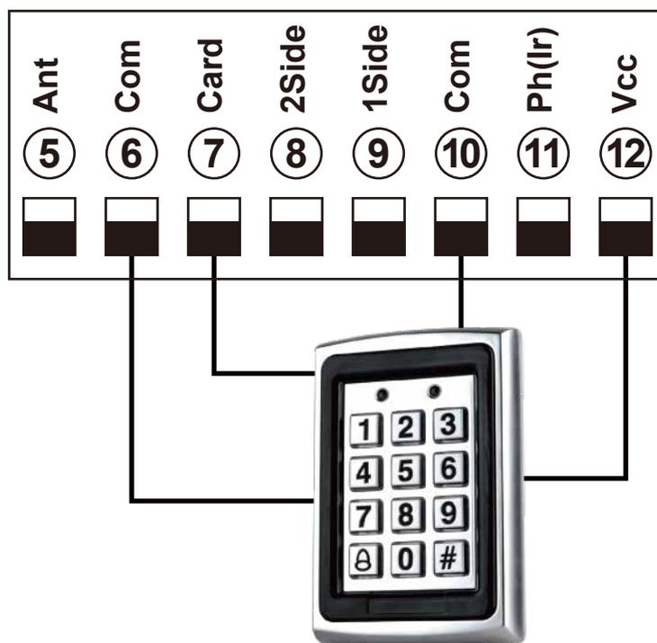
Terminal ⑫VCC and ⑩COM are used to supply power to swipe card device.
